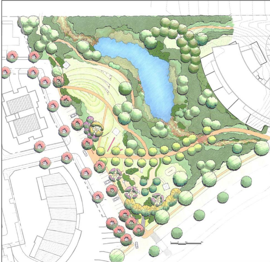
Figure 1813 Wetland park and detention basin
